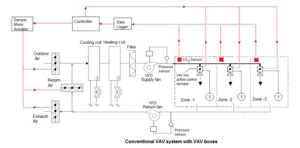
To understand how multi-zone demand ventilation control with multiple CO<sub>2</sub> sensors works, let's consider an example.
