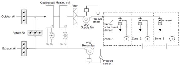
Conventional VAV system with VAV boxes
