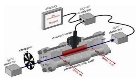
The sensor accuracy can be affected by vibration and atmospheric pressure changes but these are non-sensitive to dirt and dust.
