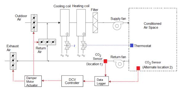
CAV SYSTEM WITH CO2 CONTROLLED VENTILATION
