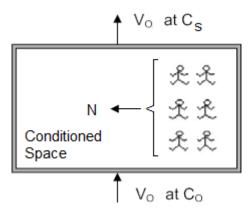
A steady-state mass balance on the CO<sub>2</sub> entering and leaving the zone gives:
