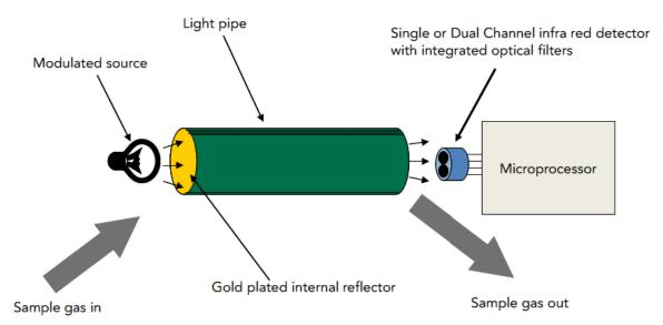
The main components of a commercial sensor are an infrared source (lamp), a gas cell/path, a wavelength selection device, and some optical components (lenses or more usually mirrors) to couple the radiation from the source through the gas cell to the detector. The sensor accuracy can be affected by the accumulation of particles in the sensor and the aging of the light source.
